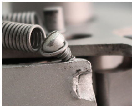
FIG. 6 Damaged Screw and Housing due to Self-Ratcheting
